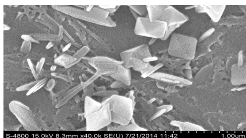
SEM micrograph of prepared \text{CoFe}_2\text{O}_4 thin film
