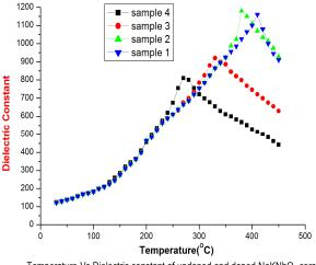
Temperature Vs Dielectric constant of undoped and doped NaKNbO ceramics
