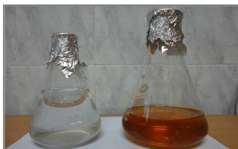
Photograph showing change in color before and after adding aqueous Curcuma caesia extract to AgNO 3
