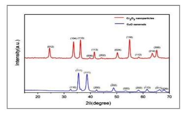
XRD spectrum of CuO-nanorods; and Nano-Cr<sub>2</sub>O<sub>3.</sub>
