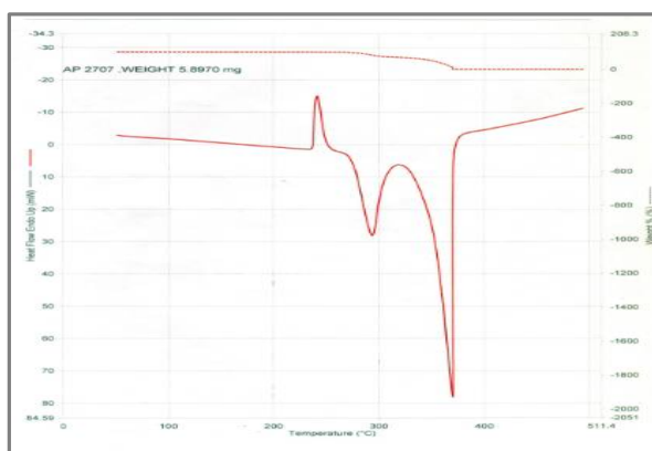
TG – DSC Curves of AP Batch No. 2707.
