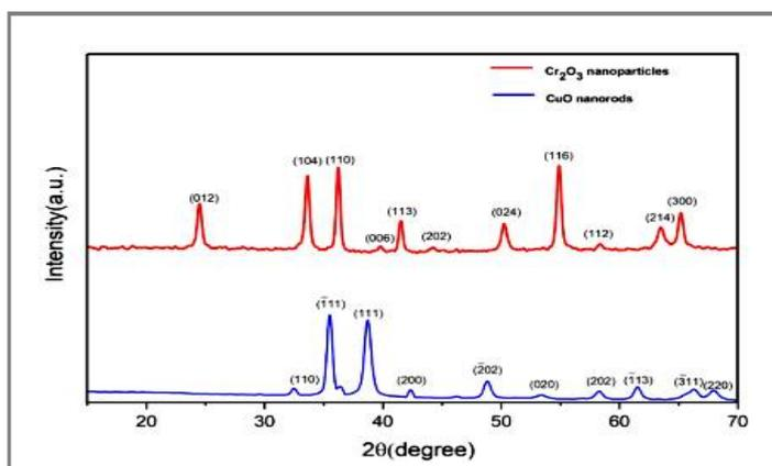
XRD spectrum of CuO-nanorods; and Nano- $\text{Cr}_2\text{O}_3$ .
