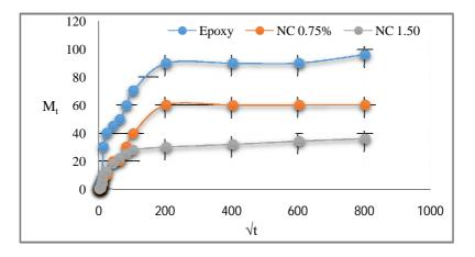
Sorption kinetics of epoxy specimens for moisture absorption for the epoxy and the epoxy filled with 0.75wt and 1.5 wt. % of nanoparticles in an atmosphere with 91% during moisture absorption.
