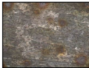
Fig 9. Photo micro graph of MS in the presence of H 2 SO 4
