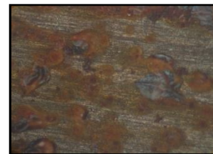
Fig 10. Photo micro graph of MS in the presence of BH
