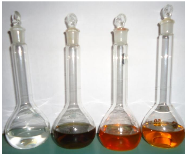
Figure 9 The colorimetric colour change on mixing of EDIMD with metals (From right to left: only EDIMD, EDIMD+Mn(II), EDIMD+Fe(III) and EDIMD+Co(II)).
