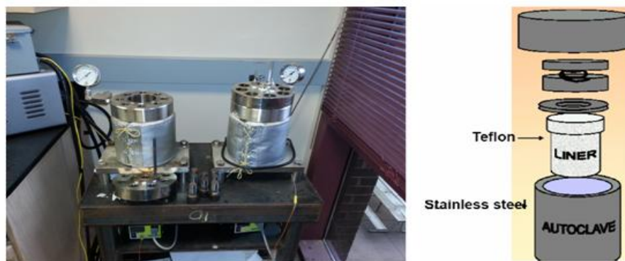
Fig.(1): Schematic of Autoclave Parr (Manufactured locally in Georgia Tech.).
