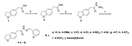
Experimental Conditions: a) EtOH, Conc; H<sub>2</sub>SO<sub>4</sub>, 12 h; b) NH<sub>2</sub>NH<sub>2</sub>.H<sub>2</sub>O, methanol, reflux, 50°C, 5 h; c) benzaldehydes **a-j**, ethanol, 45-50°C, 1 h.
