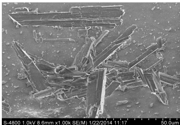
Fig 14. SEM analysis for Zeolite+Zn(II)
