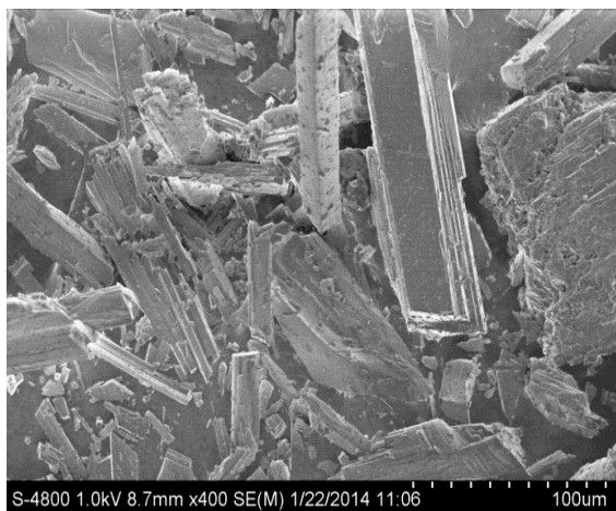
Fig 12. SEM analysis for Natural Zeolite
