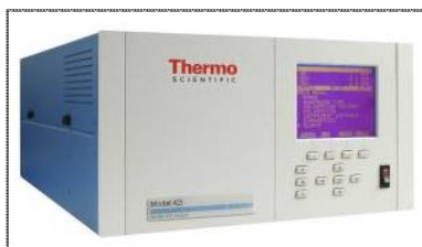
Figure 3. SO 2 analyzer (Thermo Fischer Scientific Model 43i).
