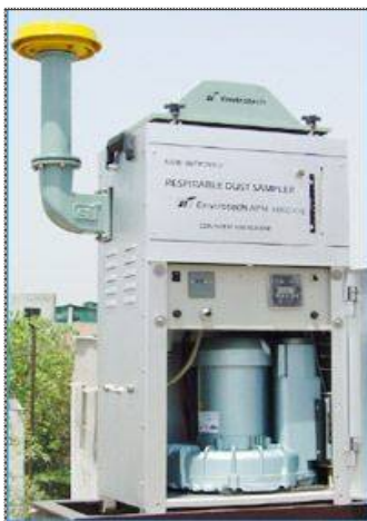
Figure 2. PM 10 Sampler (Envirotech Model APM 460 BL).
