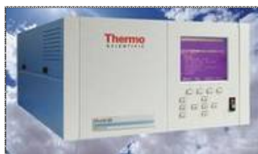
Figure 4. NO 2 analyzer (Thermo Fischer Scientific Model 42i).
