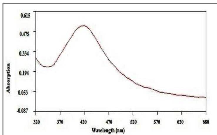
Figure 2. Confirmation of formation of AgNPs at 72 h via UV-Vis spectra at 418 nm wavelength.
