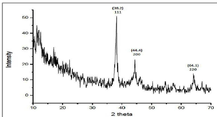
Figure 4. X-Ray Diffraction pattern of biogenic silver nanoparticles showing characteristics peaks centered indexed to the crystalline planes (111), (200) and (220) of face centered cubic silver.
