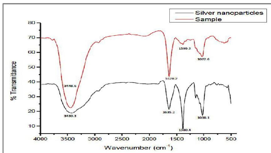
Figure 3. Fourier Transform Infrared spectrum of biogenic silver nanoparticles.
