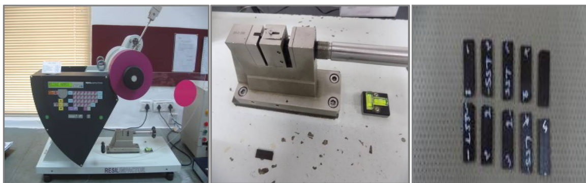
Figure 2. The Impact Specimen of PP/SEBS/Neem wood flour after test.
