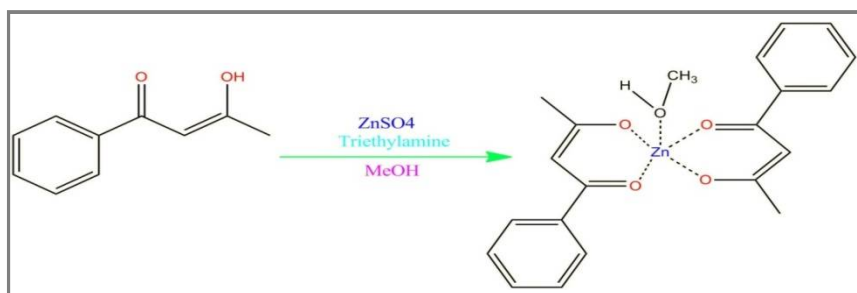
Scheme 1. Reaction pathway of (Z)-3-hydroxy-1- phenylbut-2-en-1-one Zn(II) complex.
