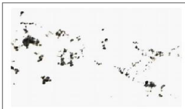
Figure 4. TEM micrograph of AgNPs synthesized using Curcuma longa leaves extract.
