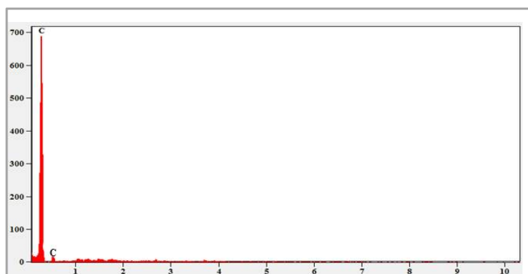
Figure 11(B). EDAX spectra of graphite Electrode.
