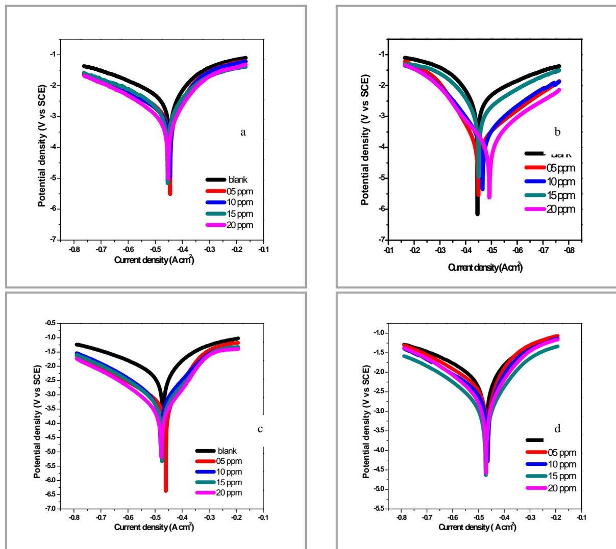
**Figure 1.** Potentiodynamic polarization (Tafel) curves for mild steel in 1N HCl solution in the absence and presence of different concentration of TG extracts of (a) leaves (b) barks (c) fruits (d) seeds.
