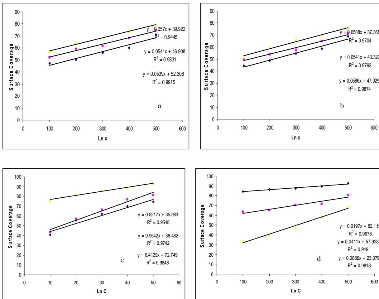
**Figure 4.** Temkin adsorption isotherm plot for mild steel in 1N HCl containing different concentration (a) leaves, (b) fruits, (c) barks, (d) seeds of the extract.
