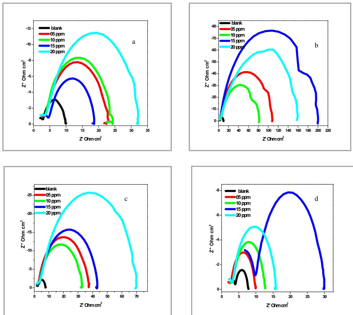
**Figure 2.** Nyquist plots for mild steel in 1N HCl acid solution without and with presence of different concentration of TG extract of (a) leaves (b) bark (c) fruits (d) seeds
