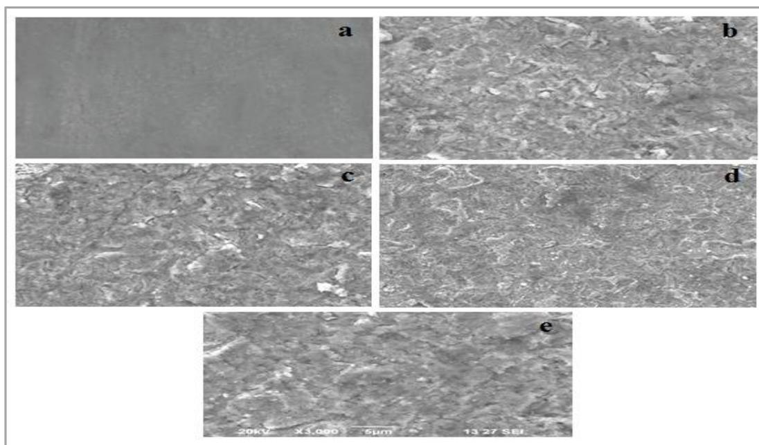
**Figure 3.** SEM image of the surface of mild steel after immersion for 24 hrs in 1N HCl solution (a) blank and in the presence of an optimum concentration of the plant extracts from (b) leaves (c) bark(d) fruits and (e) seeds.
