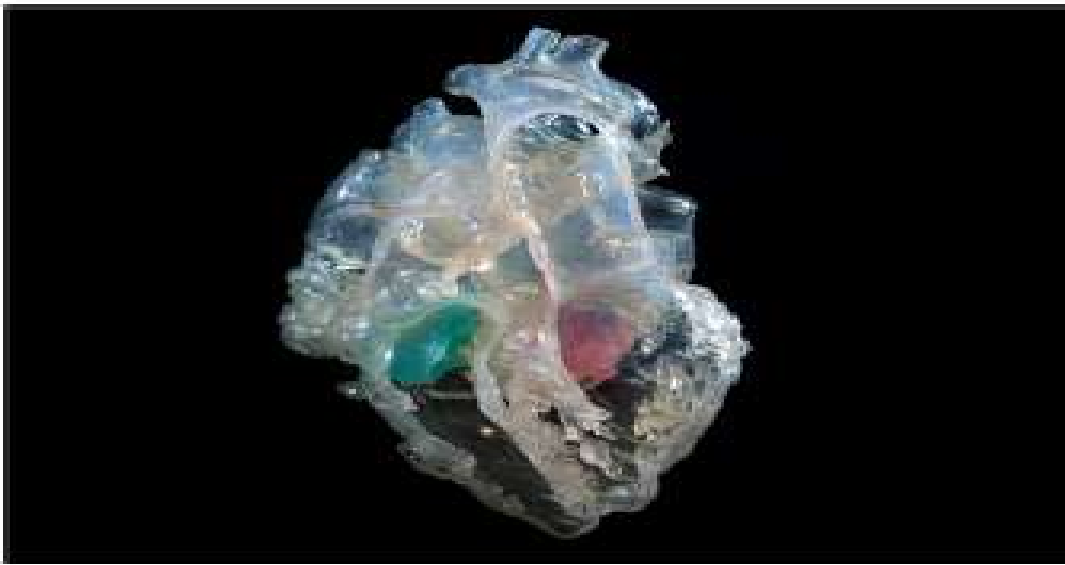
Model of the heart and major arteries using a polyjet 3D printer
